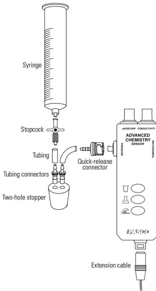
2. Connect the pressure sensor and temperature sensor to the data collection system and start a new experiment. Display the pressure on the  $y$ -axis of a graph and time on the  $x$ -axis
