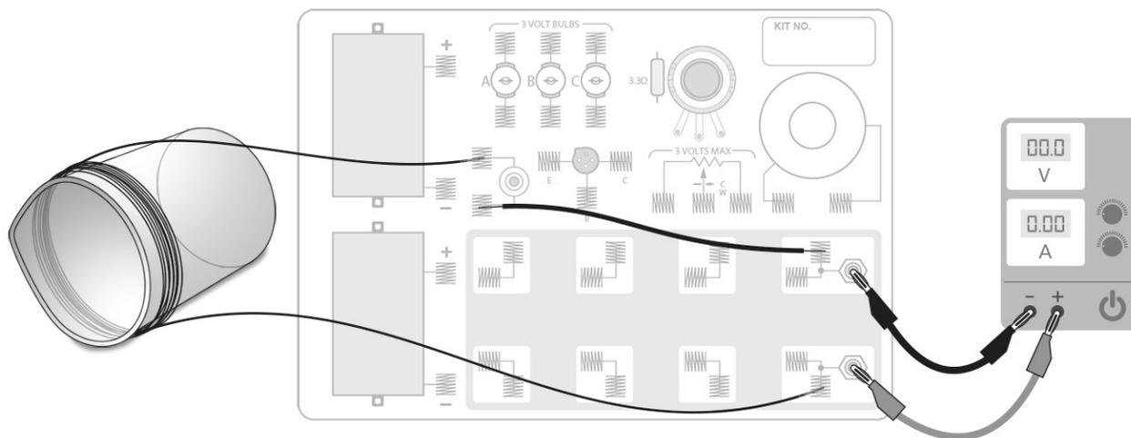
3. Turn the power supply on, press and hold the switch on the circuit board, and adjust the power supply so that 0.50 A of current is output to the coil. Release the switch every few seconds and after the adjustment is complete.
