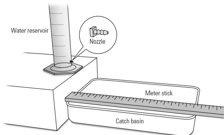
*NOTE: Unless you are absolutely certain about the path of the water stream, you may want to open the nozzle or hole and let a small amount of water out to properly align the meter stick with the stream; however, if you do so and the water level in the reservoir falls close to or below the highest graduation mark, add more distilled water to bring the water level 2 cm to 3 cm above the graduation.*
