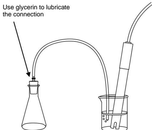
11.  Thoroughly rinse the pH sensor with distilled water.
