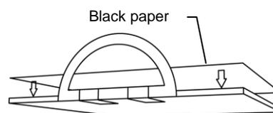
The temperature of the solar energy collection panel will increase at all three angles because the black paper absorbs the sun rays. The change in temperature will increase as the angle of insolation increases because the incoming solar radiation is more intense. Therefore the solar energy collection panel at 90° will have the greatest change in temperature.
