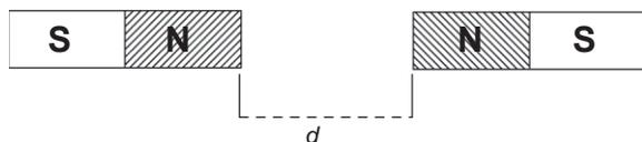
3. If each magnet alone produces an axial magnetic field strength of  $0.25\text{ T}$  at a distance  $d/2$ , what value would your magnetic field sensor read at distance  $d/2$  if the north and south poles were facing each other a distance  $d$  apart?
