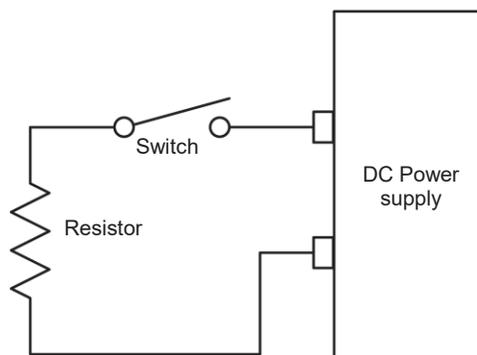
4.  Connect the voltage sensor across the resistor, and then connect the current sensor in series with the resistor and switch. Be sure the switch is open.
