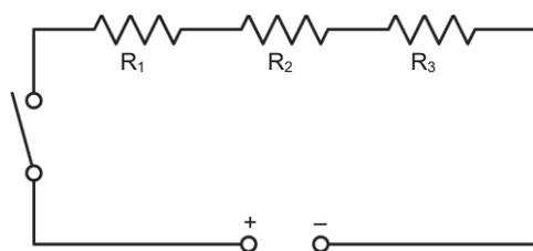
**14.**  Use the series circuit that you have created to determine if the behavior of a series circuit is Ohmic. Ensure the sample rate on your data collection system is set to 10 samples per second.  $\diamond^{(5.1)}$
