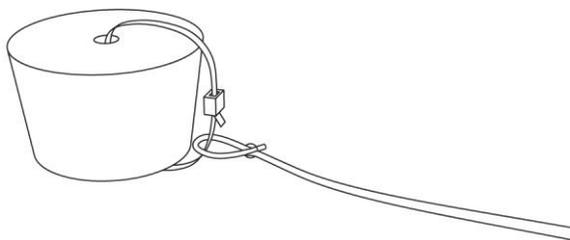
11.  Measuring from the center hole of the stopper (approximately the center of mass), mark the string at 1.0 meter from the stopper's center of mass. Record the radius in Table 1 in the Data Analysis section.
