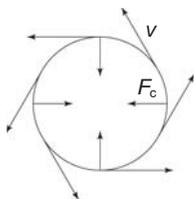
In this experiment, you will conduct several short investigations examining how the object's mass influences the period of a revolution under a constant force and constant radius. You will also examine how changing the radius of the circular path affects the period of a revolution while the object's mass and applied force are held constant. In the final investigation, you will vary the applied force to determine the effect on the period of a revolution when holding the radius and mass constant.
